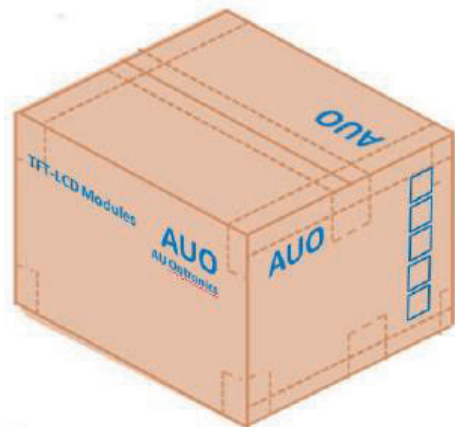
Carton bottom be closed by tape, and then put EPE Cushion and esd bag into the carton.
